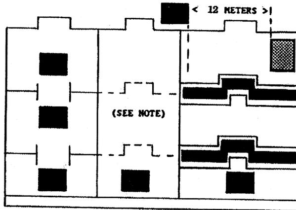
NOTE: One of the two decks must be resistant to fire and liquid.
