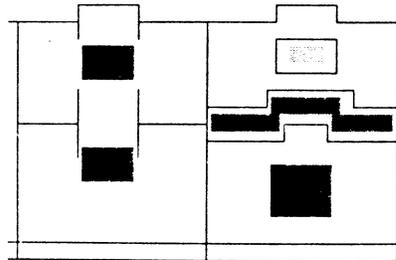
(iv) *“Separated by a complete compartment or hold from”*: Either a vertical or horizontal separation. If the intervening decks are not resistant to fire and liquid, then only a longitudinal separation (i.e., by an intervening complete compartment or hold) is acceptable. For “on deck” stowage, this segregation means a separation by a distance of at least 12 m (39 feet) horizontally. The same distance must be applied if one package is stowed “on deck”, and the other one in an upper compartment.
