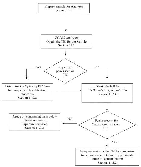
Figure 1. Schematic Flowchart for Qualitative Identification
