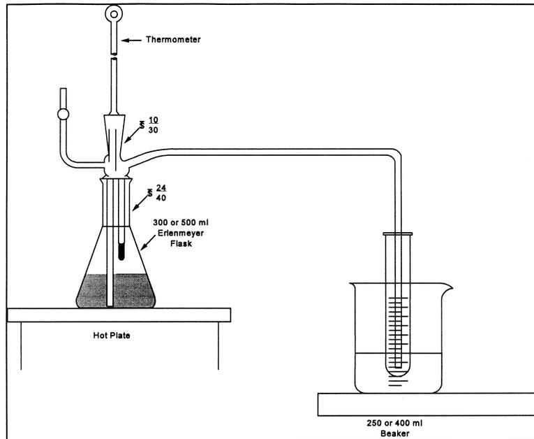
Figure 108C-1. Distillation Apparatus.
