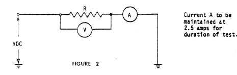
b. Operate the circuit with a regulated power supply of 14.0  $\pm$ .5 volts DC connected to the primary at an ambient temperature of 70 °C (158 °F) at 1750  $\pm$ 50 distributor rpm for a duration of 200 hours. After each 50 hour interval, run the distributor for 5 minutes with one open-circuit spark gap instead of a 12KV gap.
