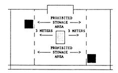
(iii) "Separated From": In different compartments or holds when stowed under deck. If the intervening deck is resistant to fire and liquid, a vertical separation (i.e., in different compartments) is acceptable as equivalent to this segregation. For "on deck" stowage, this segregation means a separation by a distance of at least 6 m (20 feet) horizontally.
